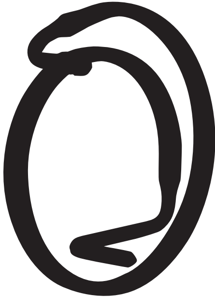
HEISE multi-coiled Bourdon tube
